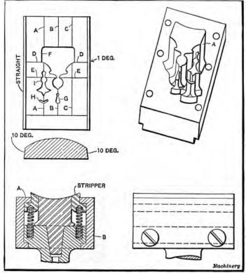
Fig. 12. Perforating Punch and Die
